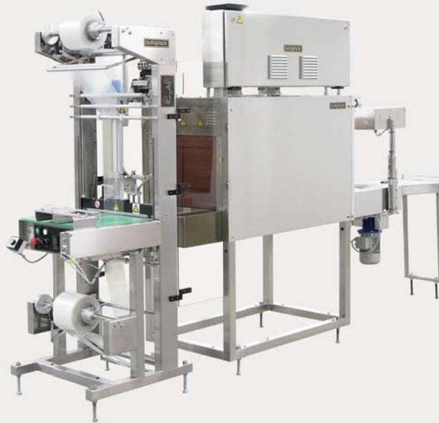
Autopack SSO is a Semi-Automatic Bundle Shrink Wrapper particularly suited for low speed application and/or contract packaging when product size, collation change many times per day. Product collation and pushing through the film is by operator, pneumatic pusher optional. Welding bar descends automatically only when the pusher is drawn back to home position to ensure operator safety.
