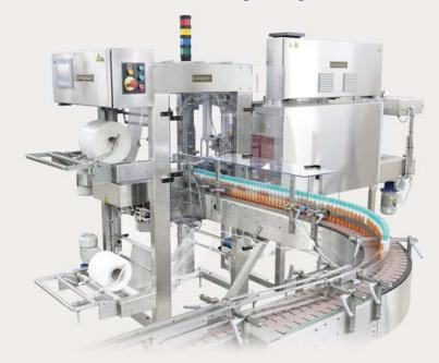
Autopack SLO Bundle Shrink Wrapper with welding bar is the ideal solution for collation and wrapping of oval shaped containers. Depending on speed and shape, the machine can be configured with or without feed screw. It is among the most compact solutions on the market, available in single, double even triple track configuration for speed up to 50 packs/min.
