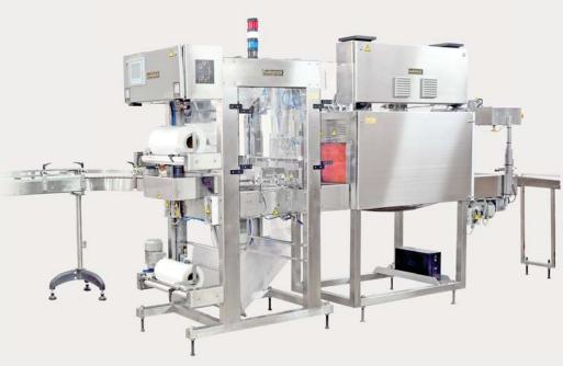
Autopack SLN with welding bar is a medium speed Bundle Wrapper designed to handle pre-loaded trays, single boxes or stacked rigid items. With its direct infeed in front of the pusher system, it is Autopack's fastest single track welding bar machine with speed up to 28 cycles/min. Autopack's compact footprint wrapper and tunnel facilitate economical use of valuable factory space.
